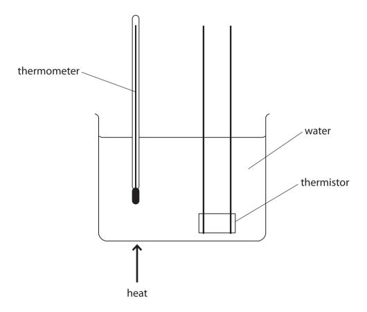
Suggest three changes to this set up that would improve the accuracy of the measurement of the thermistor temperature.
